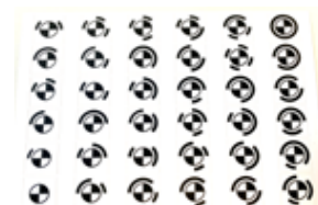
Auto-detection of coded markers (App Video: Wing Deflection Measurement in Istra4D V4.11 using point (marker) tracking)
