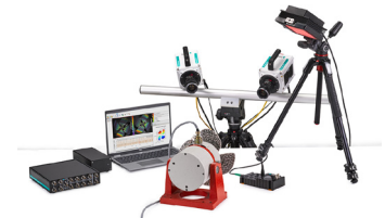
HSpeedDIC system used for deflection and ODS vibration analysis of a propeller
